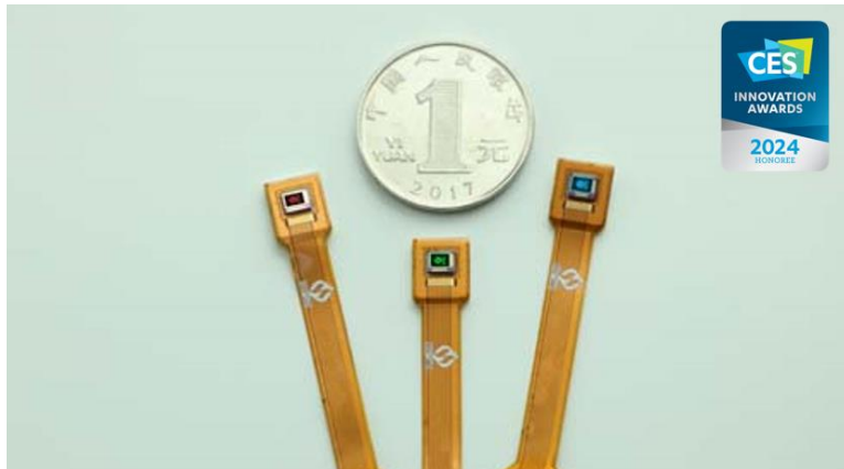
Photo 2: The “0.13” Micro-LED Display Module” developed by Sitan Semiconductor International Co Limited features an ultra-high pixel density (10,000 ppi) and provides AR/XR products with the advantages of high brightness, long lifetime, and high efficiency. It also received an Innovation Award in the “XR Technologies and Accessories” category at CES.
