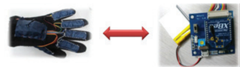
(b) Wireless smart glove system for human motion detection (Source: Prof. Inkyu Park, Korea Advanced Institute of Science and Technology)
